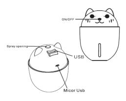
Turn counterclockwise and unscrew the top cover. Fill the tank with water (320ml). Unscrew the top cover clockwise and connect the power supply (USB cable). Click on the button (nose) to start the humidifier.
